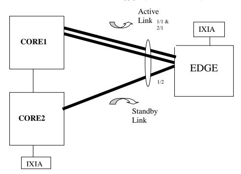
On EDGE device create the LACP linkagg group of size 4 and set port 1/2 in STANDBY mode:
